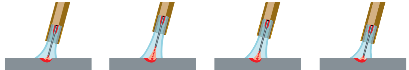
The welder can react much more easily to arising conditions by adjusting the distance of the torch.
