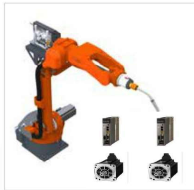
Example 2: QRH-290-6 with a combination of two rotary positioners to an L-shaped positioner
